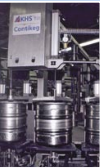
Upgraded from previously 400 kegs/h, the Innokeg Contikey line now handles 1,000 kegs/h.
