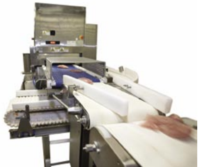
Rose Poultry has installed an Ishida IX-GA-2475 X-ray inspection system on each of its two frozen chicken fillet lines.
